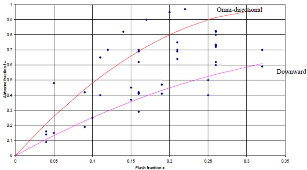
Figure 4-3 Airborne Fraction correlations in ACE from [5]
